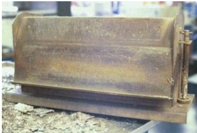
Pic. 4: Solder nozzle from modified material after 3,5 years of use
