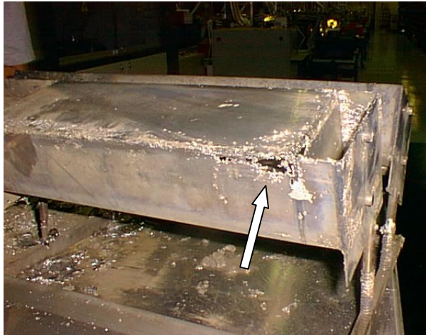
Pic. 1: Defective Pump Housing
