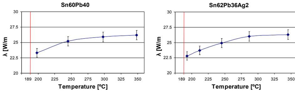
Fig. 4: Thermal conductivity of tin/lead solders (red line shows the upper region of the melting range)
