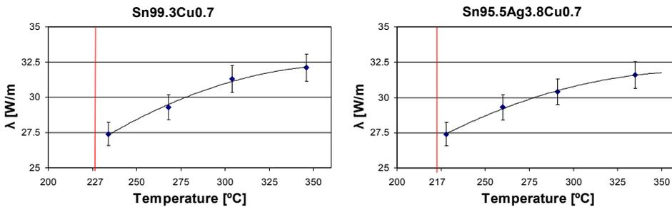
Fig. 5: Thermal conductivity of lead-free solders (red line shows the melting point – eutectic solders)
