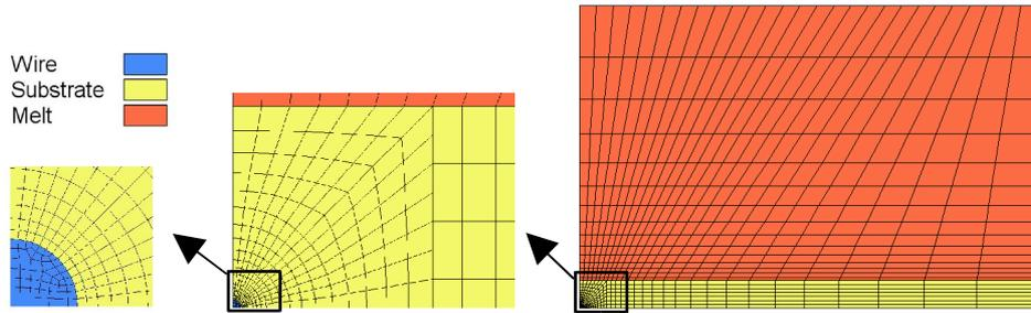
Fig. 2: Meshed 2D model of the cross-section of the sensor and melt
