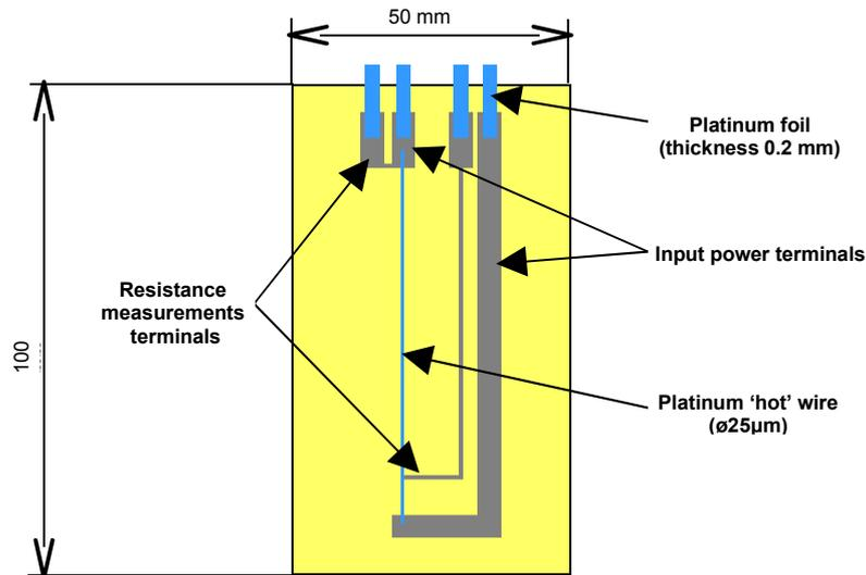
Fig. 1: Sensor (top view before covering wire and thick film pattern with alumina tape)
